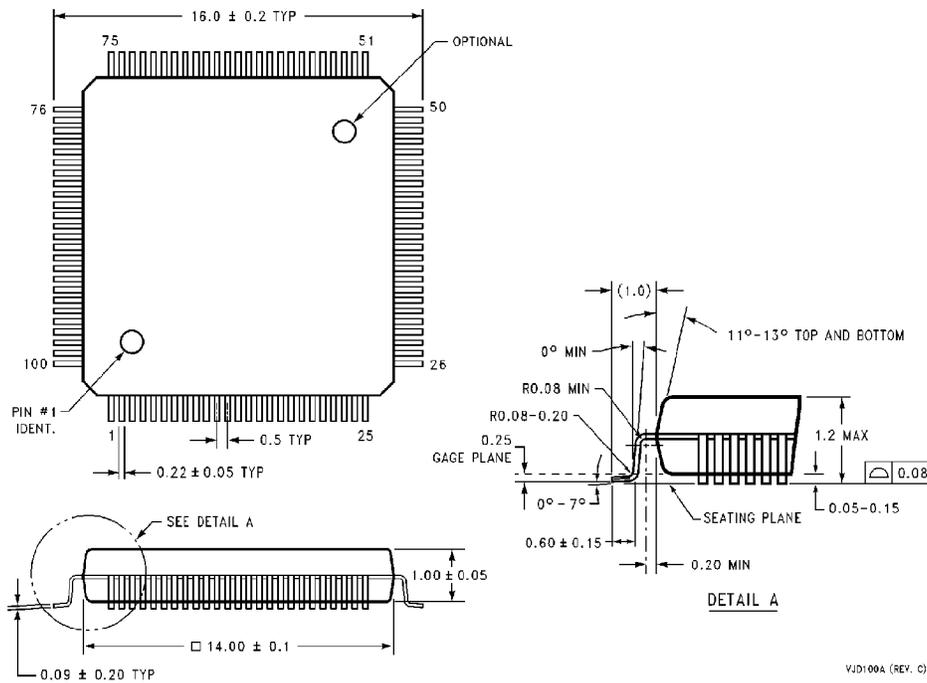
**100-Pin Thin Plastic Quad FlatPac (JEDEC) (TQFP)**
