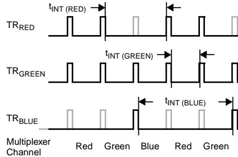
**Figure 38: 3 Channel Line Rate TR Pulse Timing**
