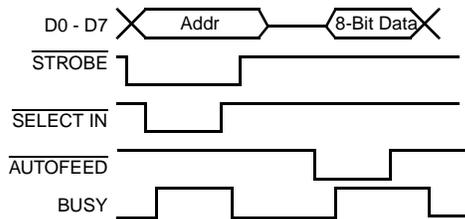
Figure 54: Reading from the Configuration Register (EPP)
