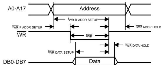
Figure 8: SRAM Write
