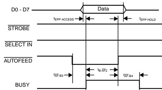
Figure 3: Parallel Port 8 Bit Data Read
